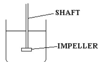
The degree of agitation is controlled by the rotational speed of impeller, by the patterns of the liquid flow and the resultant efficiency of mixing are controlled by the type of impeller, its position in the container, the presence of baffles, and the general shape of the container.
